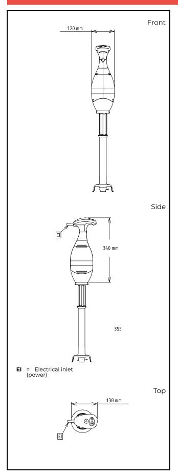
Electric Supply voltage: 220-240 V/1 ph/50/60 Hz **Electrical power max:** 0.45 kW 0.45 kW **Total Watts:** Key Information: External dimensions, Width: 138 mm External dimensions, 120 mm Depth: External dimensions, 340 mm Height: **Shipping weight:** 3.65 kg
